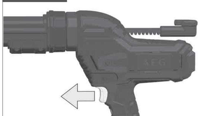
When the trigger is released, the motor will run for a short time to release the rod. This prevents a drip.
