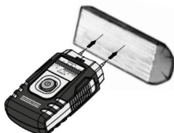
The location to be measured should be untreated, free of knots, dirt and resin. Measurements should not be made on the end faces of wood because these areas dry particularly quickly such that they produce incorrect measurement results.
